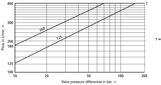
1 = Recommended flow limitation (flow velocity 30 m/s) in the valve connection ports
