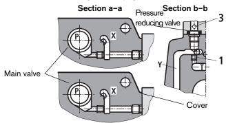
Pilot oil supply external: P closed (section a-a) internal: P open Pilot oil drain external: 1 closed
