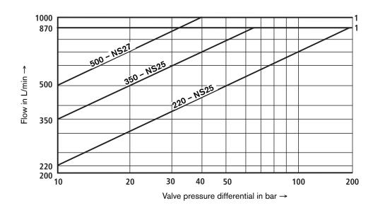
1 = Recommended flow limitation (flow velocity 30 m/s) in the valve connection ports
